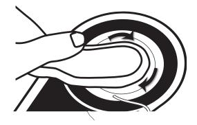
Turn it clock-wise to tighten the valve.
